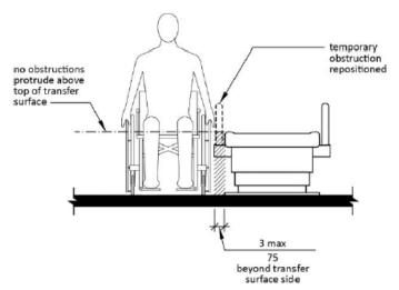
Permit up to 3-inch "gap" at/below transfer surface
